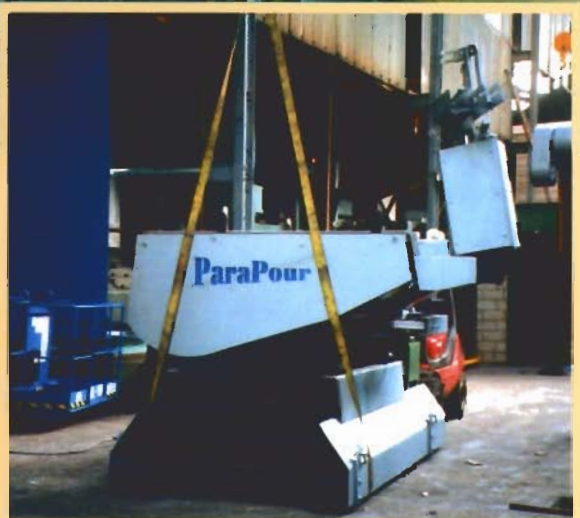
Easy installation on floor mounted rails one side of the mould line
