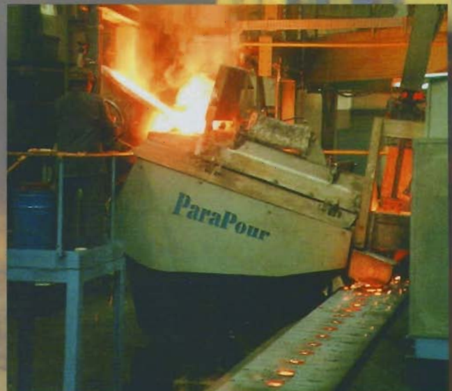
Continuous pouring during filling
