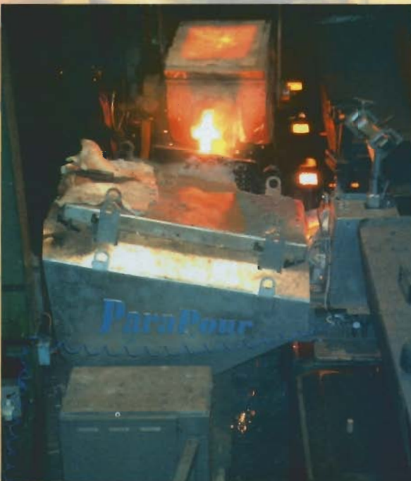
Side fill unit on large flasked line
